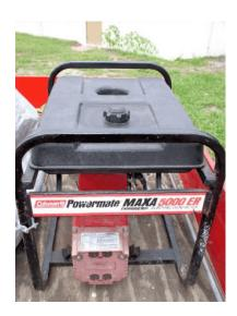
**Briggs & Stratton**, 5000 Watts, 41.6/20.8 Amps 2 - 120 volt outlets, 1 - 240 volt outlet 10 hp Briggs & Stratton, 6 qt. tank
